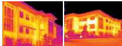
Standard Lens Wide Lens see both sides of the building at the same time from the same distance
